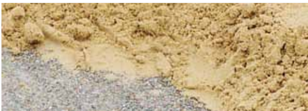
Stepping layer is loosely lying on a stable grip layer for safe and controlled sliding
