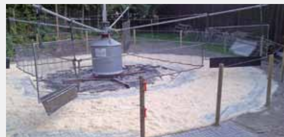
Horse walker with shock-absorbing TTE® plaster floor
